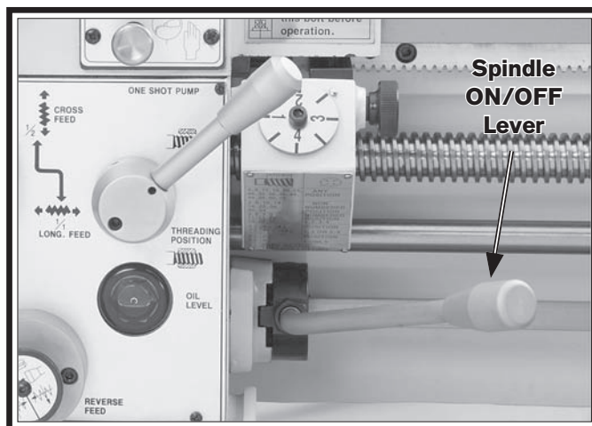
Figure 33. Spindle ON/OFF lever in the OFF (middle) position.
